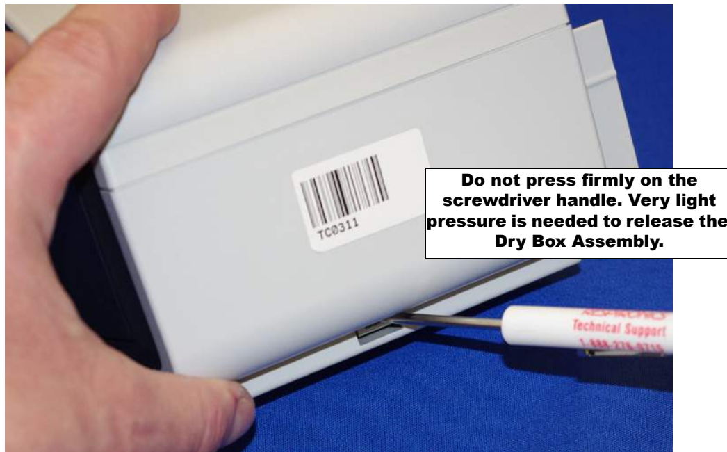
FIGURE 7-5: DRY BOX SEAL REMOVAL
