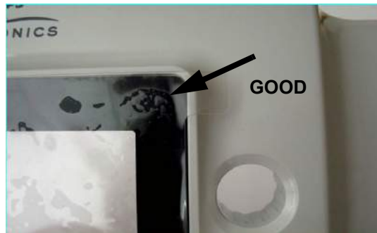
FIGURE 6-3 GOOD UI PANEL INSTALL
