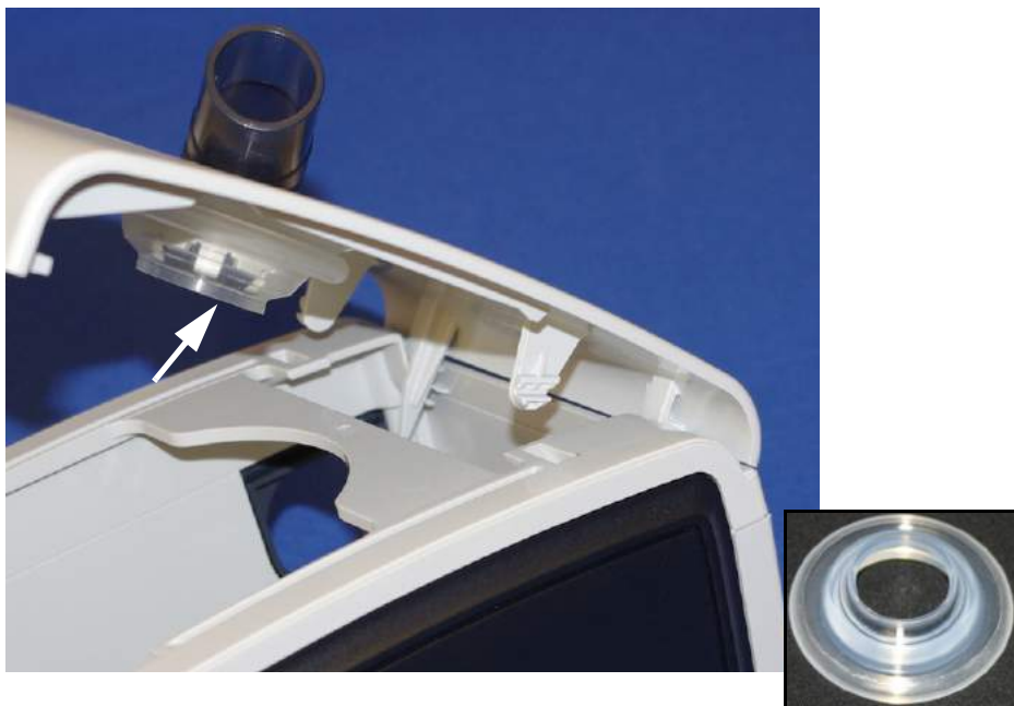
FIGURE 7-2: TANK TOP SEAL
