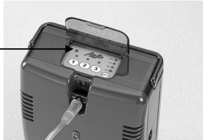
Figure 25: Indicator of Required Inspection/Service
