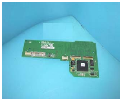
System Interconnect Board
