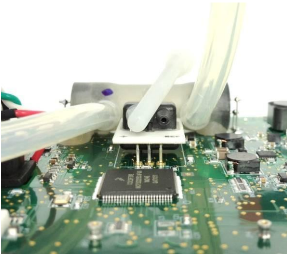
Figure 12: Pins aligned with motherboard holes
