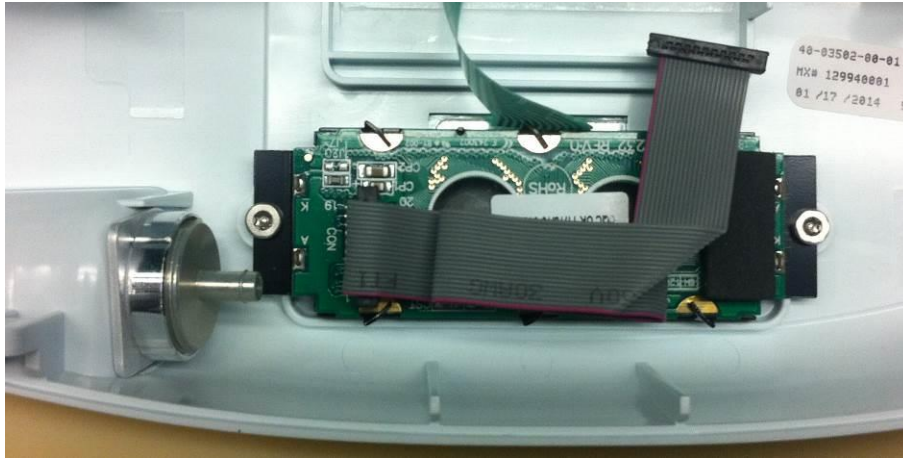
Figure 6: Orientation of LCD cable
