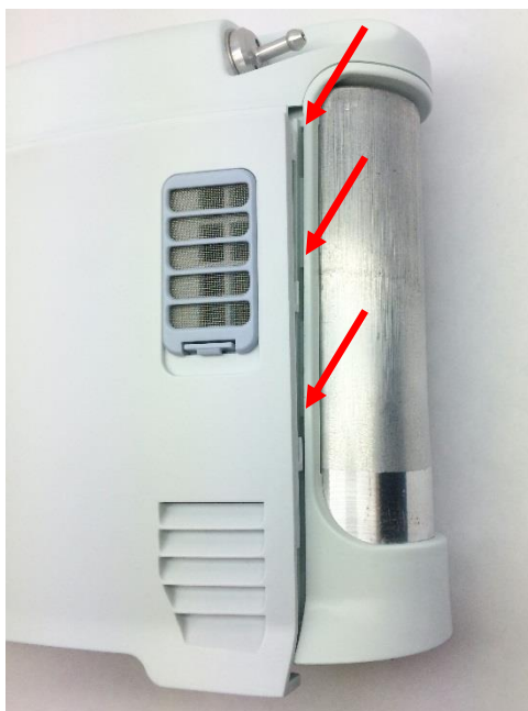
Figure 9: Housing feet and corresponding chassis grooves
