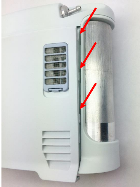
Figure 11: Housing feet and corresponding chassis grooves
