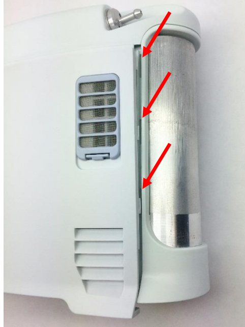
Figure 7: Housing feet and corresponding chassis grooves
