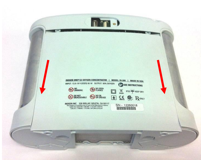
Figure 3: Direction to slide housing
