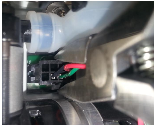
Figure 2: Detach compressor cable from motherboard
