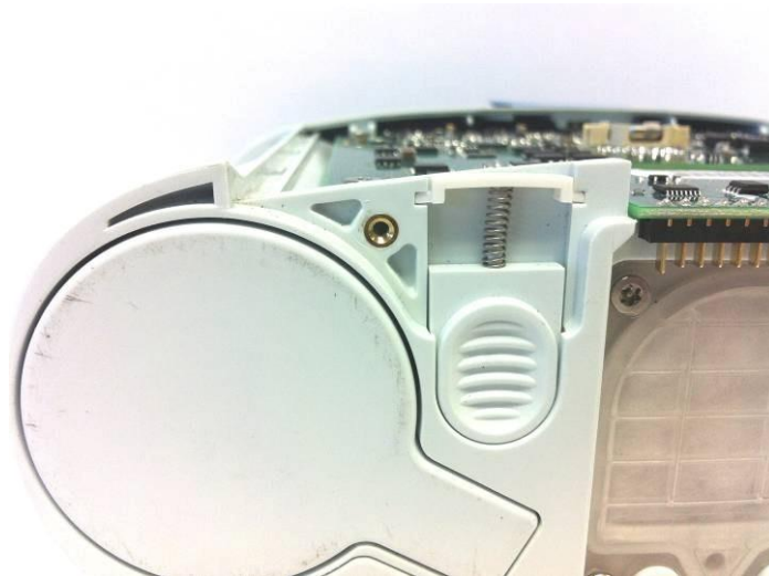
Figure 7: Properly seated spring nest and column latch
