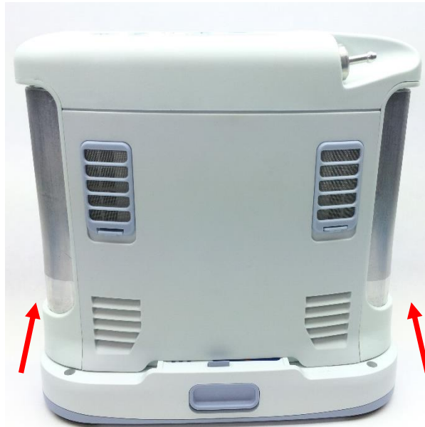
Figure 1: Direction to slide device to remove battery
