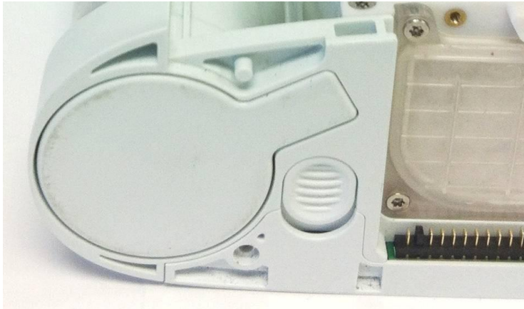
Figure 6: Correctly installed column ( Note location of column latch )
