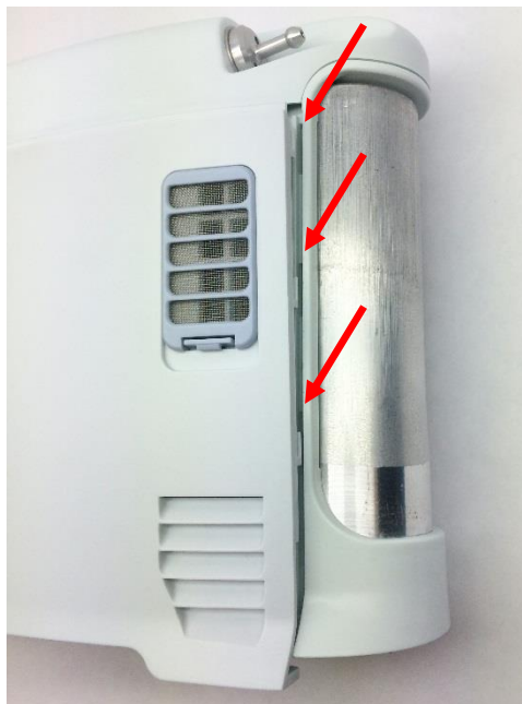
Figure 11: Housing feet and corresponding chassis grooves
