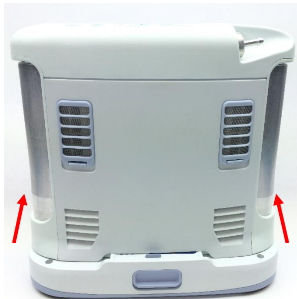
Figure 1: Direction to slide device to remove battery
