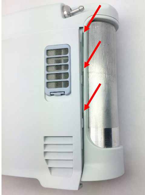
Figure 10: Housing feet and corresponding chassis grooves
