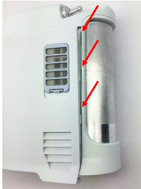
Figure 14: Housing feet and corresponding chassis grooves
