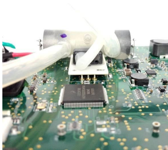
Figure 13: Fully seated breath detect
