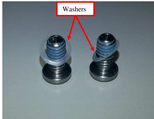
Figure 7: Torque the screws to 10 in-lbs.
