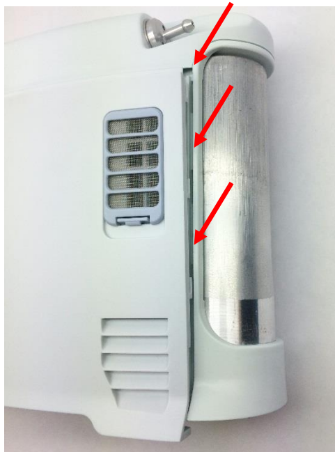
Figure 10: Housing feet and corresponding chassis grooves
