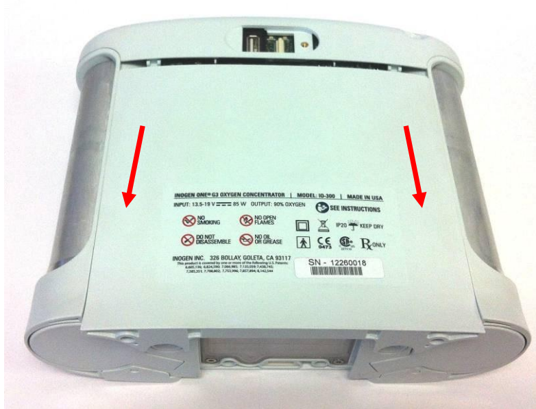
Figure 3: Direction to slide housing
