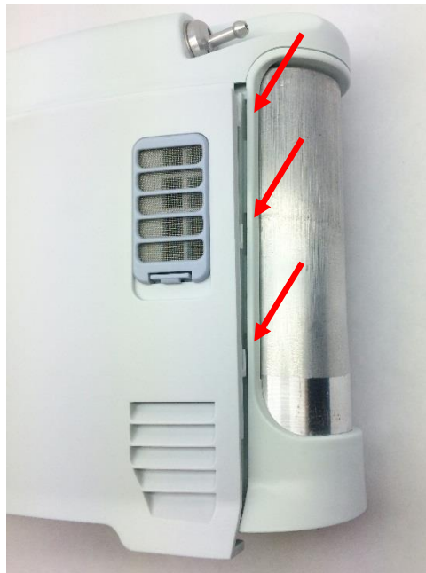
Figure 9: Housing feet and corresponding chassis grooves
