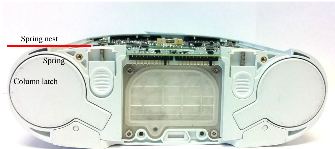
Figure 4: Column latch assembly
