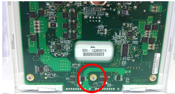
Figure 1: Location of rear filter body screw
