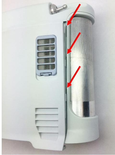
Figure 8: Housing feet and corresponding chassis grooves
