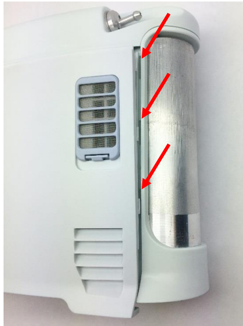
Figure 11: Housing feet and corresponding chassis grooves
