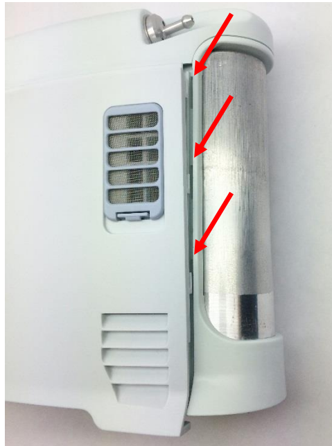
Figure 9: Housing feet and corresponding chassis groove.
