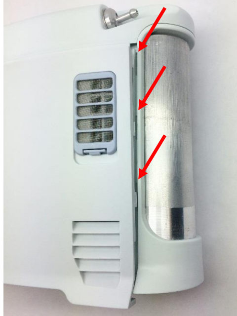
Figure 4: Housing feet and corresponding chassis grooves
