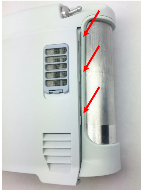
Figure 7: Housing feet and corresponding chassis grooves
