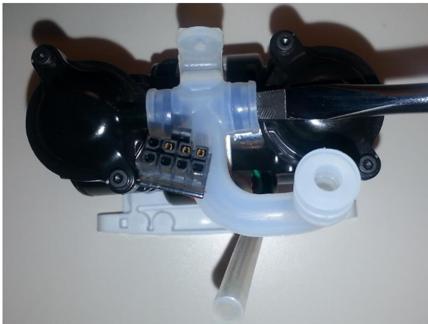
Figure 8: Remove dual feed tube from compressor
